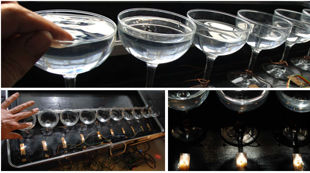
Figure 1: The poseidophone is a musical instrument in which water is the initial sound-producing medium. As with an electric guitar (chordophone) there is an electric pickup that can be acoustic, optical, or any of a variety of other forms of pickup. With this poseidophone, the glasses, with water, form very good aspheric lenses to concentrate the sun's rays (or rays from a stage light during a performance) onto high-temperature ceramic pickups that optically respond to sound waves (ripples) in the water.
